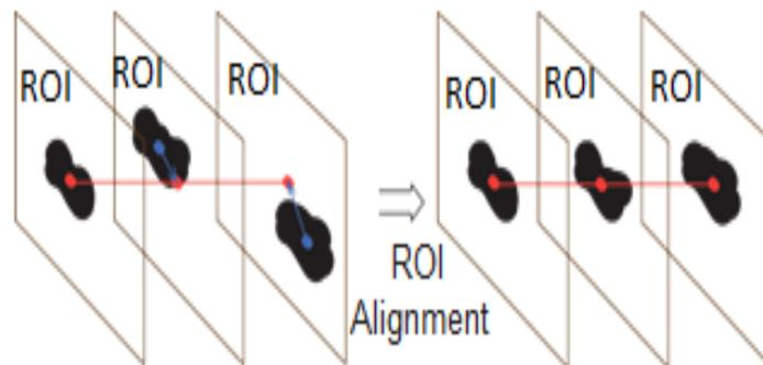
Fig.3. ROI Alignment technique to convert the image to a binary map
